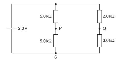
$V_1$  is the potential difference between S and P.  $V_2$  is the potential difference between S and Q.
