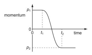
Initially, the momentum is  $p_1$  at time  $t_1$ . At time  $t_2$  the momentum is  $p_2$ .
